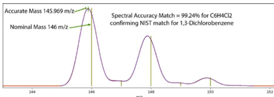
The profile mode spectral overlay of the calculated “True” MS (Blue) and the calibrated (Red) MS shows nearly a perfect match with 99.24% spectral accuracy confirming the NIST compound formula for more confident ID. This is a feature previously only available in high resolution MS.
