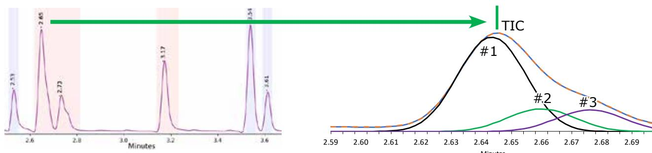
The peak at 2.65 min actually contains 3 co-eluting peaks which GC/ID deconvolves as shown. Version 2 provides improved deconvolution and, unlike conventional approaches, minimizes over fitting and eliminates false hits.
