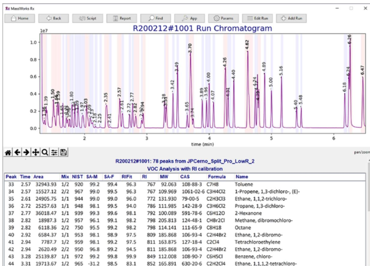
GC/ID processes an entire run in a few minutes, calculates the NIST match value (NIST) for each peak, verifies the compound formula by accurate mass/spectral accuracy via M+ (SA-M) as well as fragment ions (SA-F), and then performs retention index match (RI Fit). **These additional metrics can dramatically improve compound identification confidence.**
