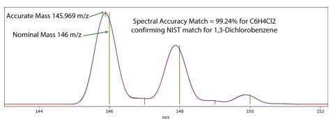
The profile spectral overlay of the calculated "True" MS (Blue) and the calibrated (Red) MS are identical to within 99.24% spectral accuracy confirming the NIST compound formula for more confident compound ID. This is a feature previously only available in high resolution MS.
