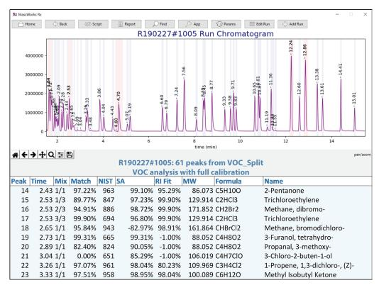
GC/ID processes an entire run in a few minutes and calculates the NIST match value (NIST) for each peak, verifies the compound formula ID by accurate mass/spectral accuracy (SA) and then calculates the peak's retention index (RI Fit). A combined (Match) value is also calculated. **These additional metrics can dramatically improve compound identification confidence.**
