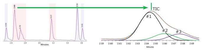
The peak at 2.65 min is actually 3 co-eluting peaks which GC/ID deconvolves as shown.
