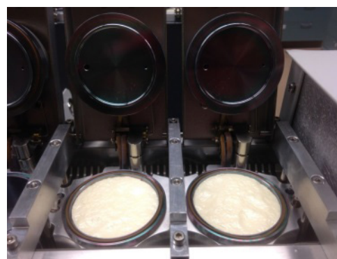
Figure 2: Generic closed-cell SPF samples in place within the \mu -CTE.
