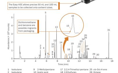
Rapid and representative sampling of meat headspace was achieved here using Markes' Easy-VOC grab-sampler. Packing the TD tubes with two hydrophobic sorbents allowed over 30 components to be analysed without interference from water. Removal of baseline interference and compound identification was carried out using TargetView software – see page 42.
