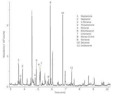
**Reactive polar analytes** such as aldehydes are successfully analysed in this yoghurt sample, thanks to the options for water management offered by Markes' TD instruments (and the inertness of the flow path). Use of a trap temperature above 0°C improves analytical reproducibility by completely avoiding problems with ice accumulation.
