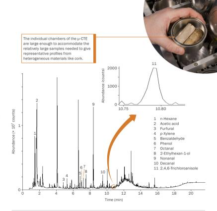
An elevated temperature was used to rapidly release the headspace from whole corks using the Micro-Chamber/Thermal Extractor (μ-CTE), leading to the detection of TCA at trace levels despite a complex background.
